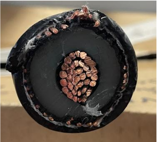
11kV XLPE cables 1980's onwards
